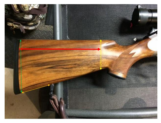
Red Line: Measure from the edge of the wood to the yellow line. The yellow line can be anywhere you want to the cuff to stop, but cannot extend past the thumb break in the pistol grip.
